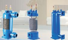
Due to the adoption of seamless titanium tube by the water side, and rigid polyvinyl chloride PVC material by the outer shell, Gree swimming pool heat pump can achieve high acid resistance, great alkali resistance, excellent corrosion resistance, and low fluid resistance, which makes it more suitable for the heat exchange of frequently-disinfected swimming pool water.
