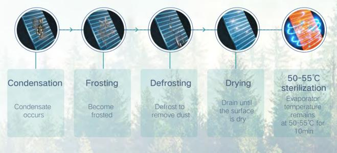
Note: Cooling-only units have four steps----condensation, frosting, defrosting and drying; cooling and heating units have five steps----condensation, frosting, defrosting, drying and 50-55°C sterilization.
