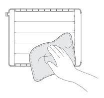
6. Cleaning of standard collector: dip the standard collector in the water for about 30 minutes, and then use cloth to wipe it up and dry it by air (or by blower); please ensure that the inner components are dry without residual water. Note: you can add proper detergent in the water when cleaning the unit to strengthen the cleaning effect.
