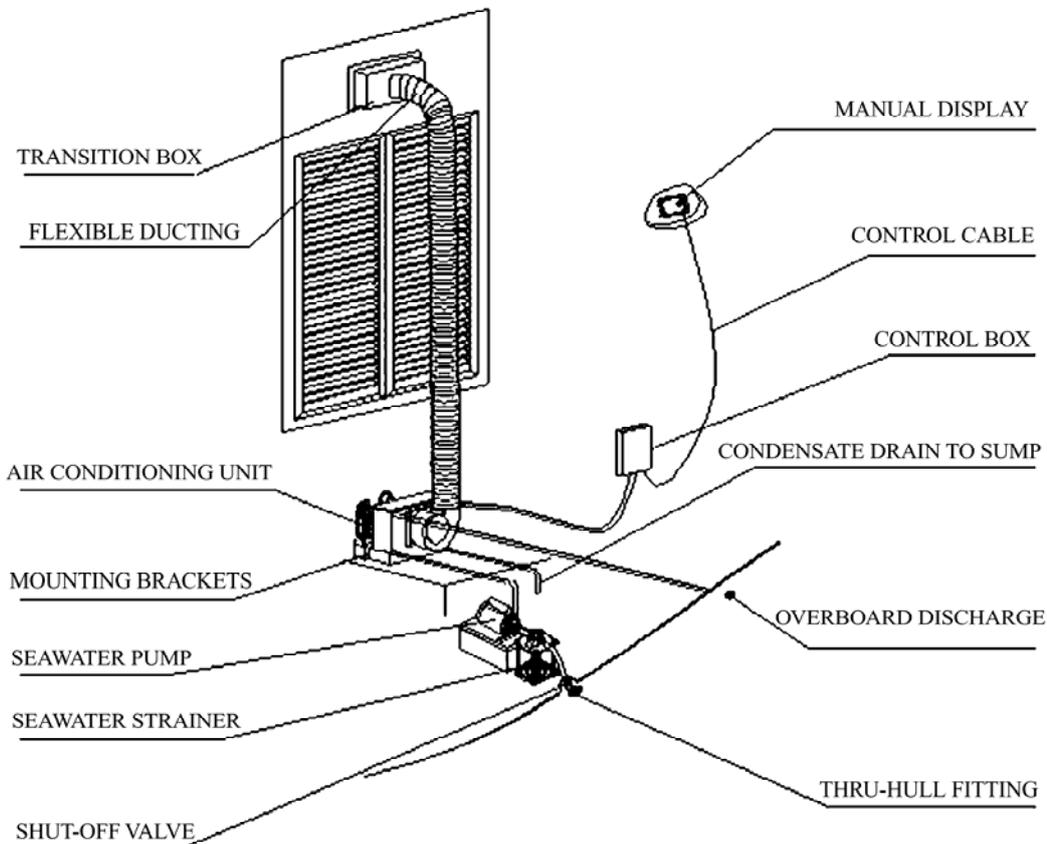
The unit should be installed as low as possible, **BUT NEVER IN THE BILGE OR ENGINE ROOM AREAS, ENSURE THAT THE SELECTED LOCATION IS SEALED FROM DIRECT ACCESS TO BILGE AND/OR ENGINE ROOM VAPORS.** Installing the unit as low as possible (such as under a V-berth, dinette seat or bottom of a locker) and ducting the supply air as high as possible, creates an ideal airflow condition. This type of installation will prevent short or premature cycling.
