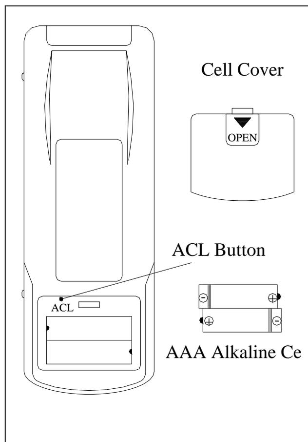
1. Slide the cell cover downward to take out the worn cells. Replace the worn cells. (Note to the correct polarity).
